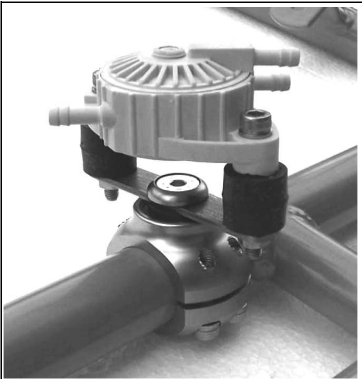
Foto of the frame with the section of the support for the fuel pump (fuel pump mounted)
